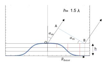
Maximum optical path difference of rays is 2h for central maximum.
