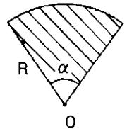
$$ĐS : a) OG = \frac{2R}{\pi} \quad b) OG = \frac{4R}{3\pi}; \quad c) OG = \frac{2R \sin \frac{\alpha}{2}}{\alpha}$$
